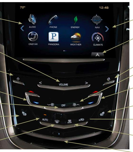
The controls use capacitive technology – simply touch the icon/text to access a feature or adjust a function
